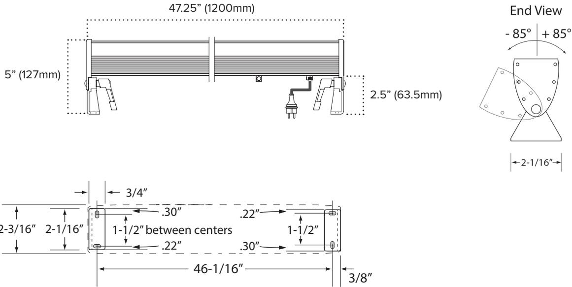
**Mounting Hole Locations of Mounting Brackets**
